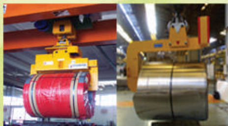
Coil Lifting Equipment
