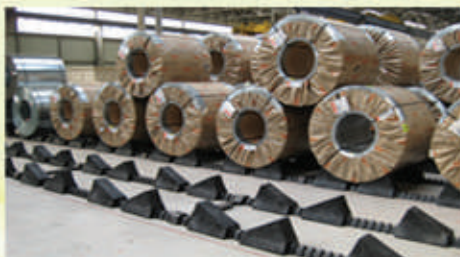
Coil Storage Equipment
